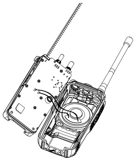
**Figure 3****Assembling the Aluminum Chassis**
